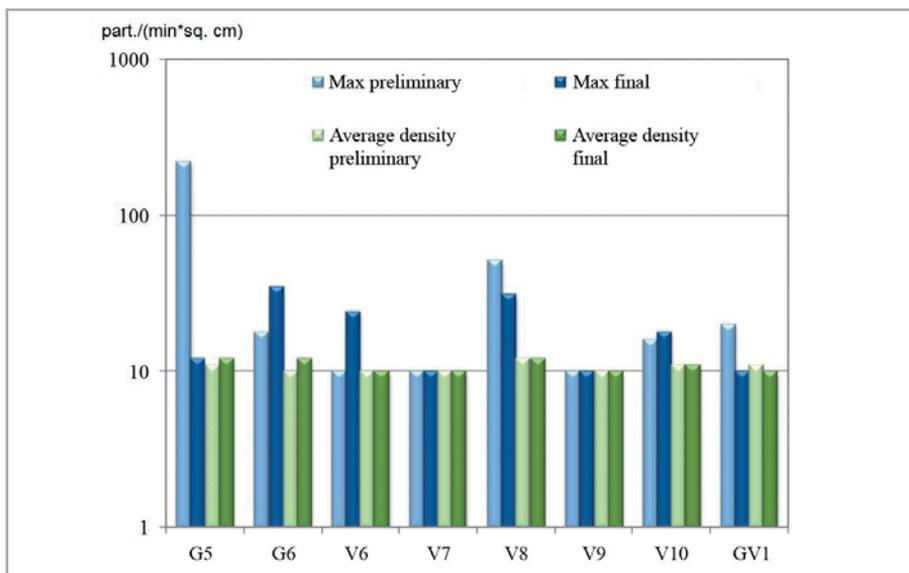
**Figure 44.** Maximal values and average density of flux of  $\beta$ -particles registered in the preliminary and final tunnel inspections
