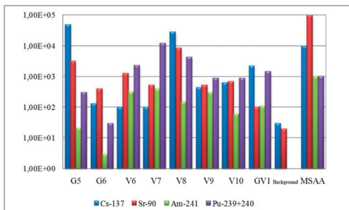
**Figure 23.** Maximal values of radionuclides specific activity for the period of preliminary inspection of the tunnels, Bq/kg
