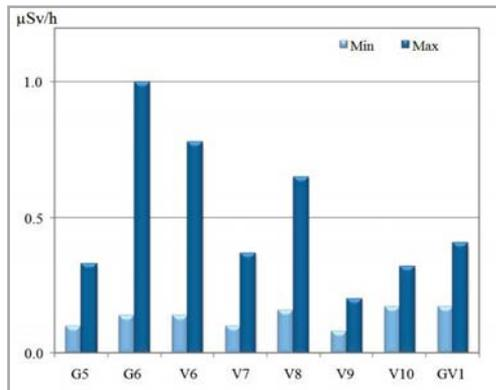
**Figure 40.** Maximal and minimal measured EDR values on the territory of the near-portal areas after completion of conservation works
