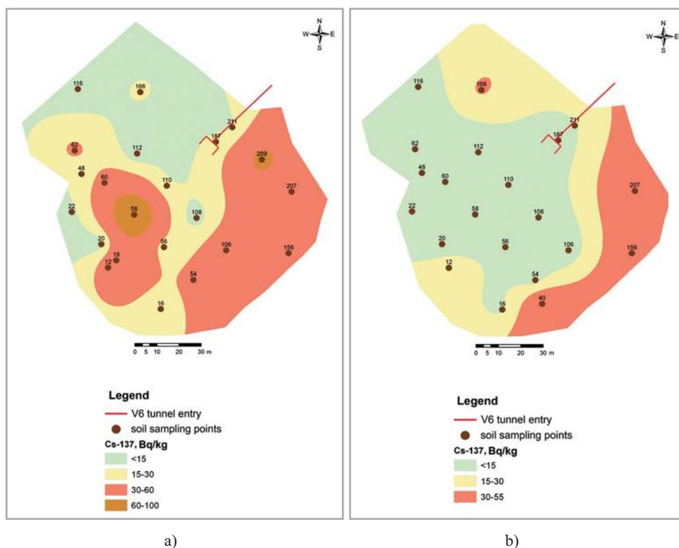
**Figure 32.** Schematic maps of  $^{137}\text{Cs}$  distribution on the territory of the near-portal area of tunnel V6 during preliminary (a) and final (b) inspections
