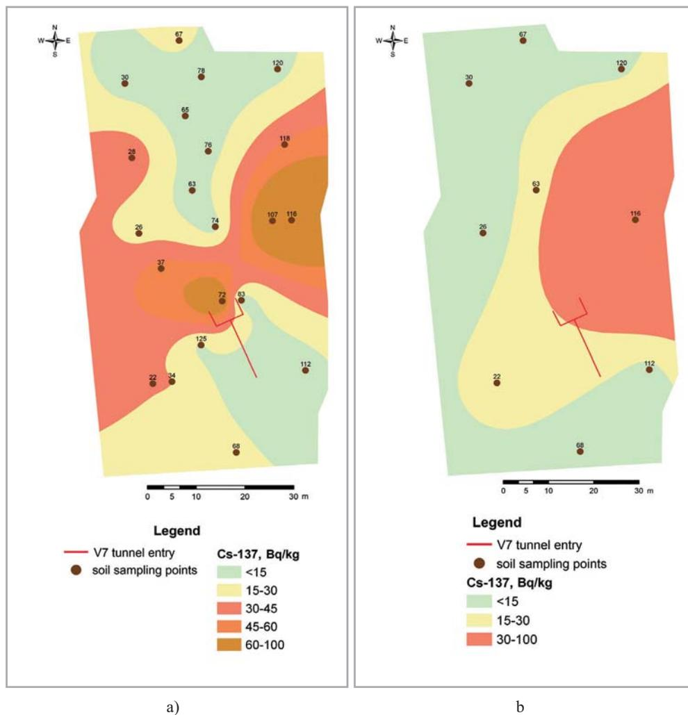
**Figure 34.** Schematic maps of  $^{137}\text{Cs}$  distribution on the territory of the near-portal area of tunnel V7 during preliminary (a) and final (b) inspections
