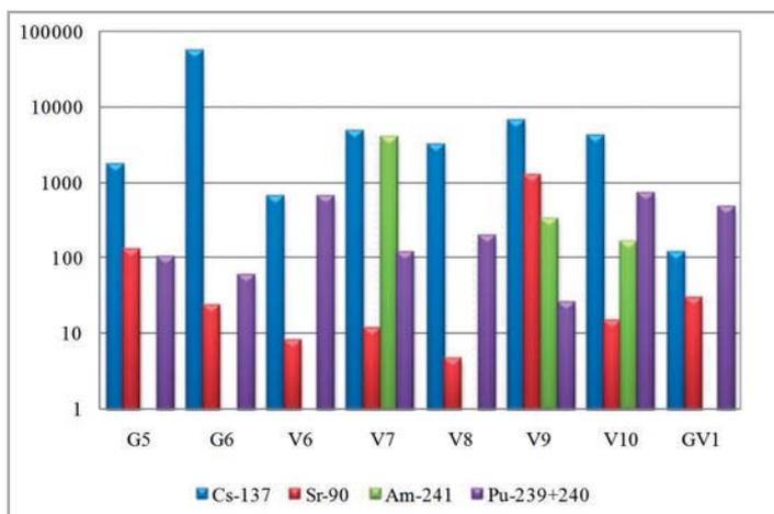
**Figure 4.** Maximal values of radionuclide specific activities after conservation works registered during final inspection of tunnels in 1999, Bq/kg.
