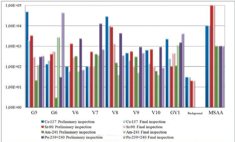
**Figure 45.** A comparison of maximal values of radionuclide specific activities registered in the preliminary and final inspections of the near-portal tunnel areas, Bq/kg
