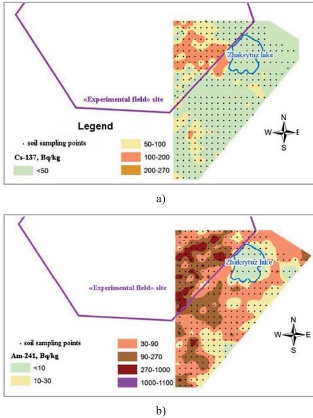
Figure 4. A schematic map of  $^{137}\text{Cs}$  (a) and  $^{241}\text{Am}$  (b) distribution in the surface layer
