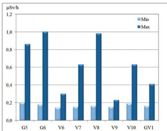
Figure 5. Maximal and minimal EDR values during the preliminary tunnel inspection
