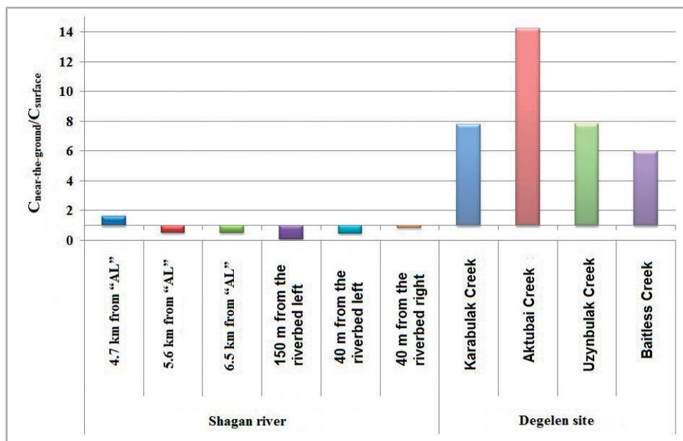
**Figure 10.** Average ratios of the tritium concentration in the near-the-ground layer to the tritium concentration in the surface layer of the snow cover
