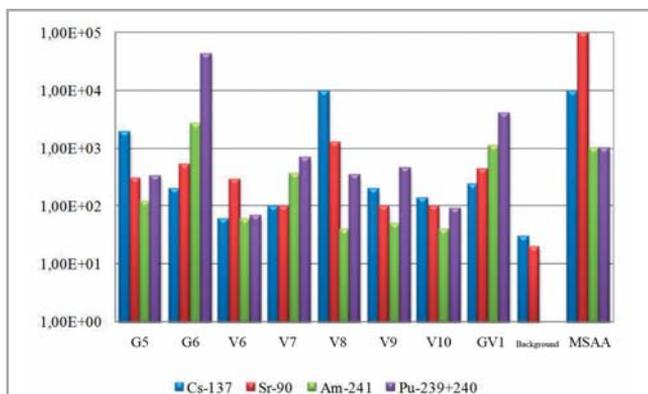
**Figure 42.** Maximal values of the radionuclides specific activities during final inspection of the tunnels, Bq/kg
