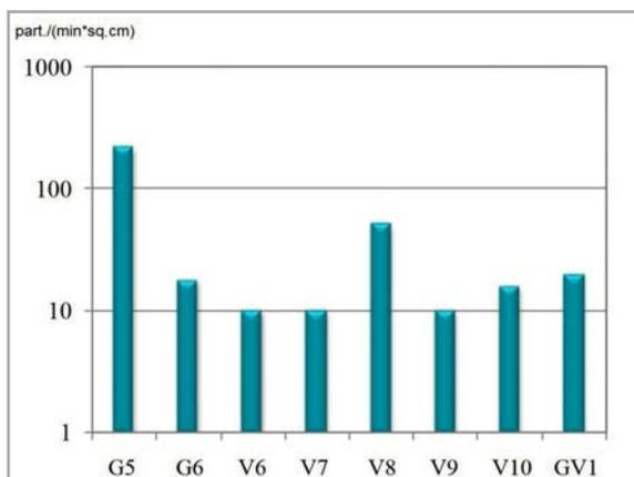
Figure 6. Maximal values of the  $\beta$ -flux density during the preliminary tunnel inspection
