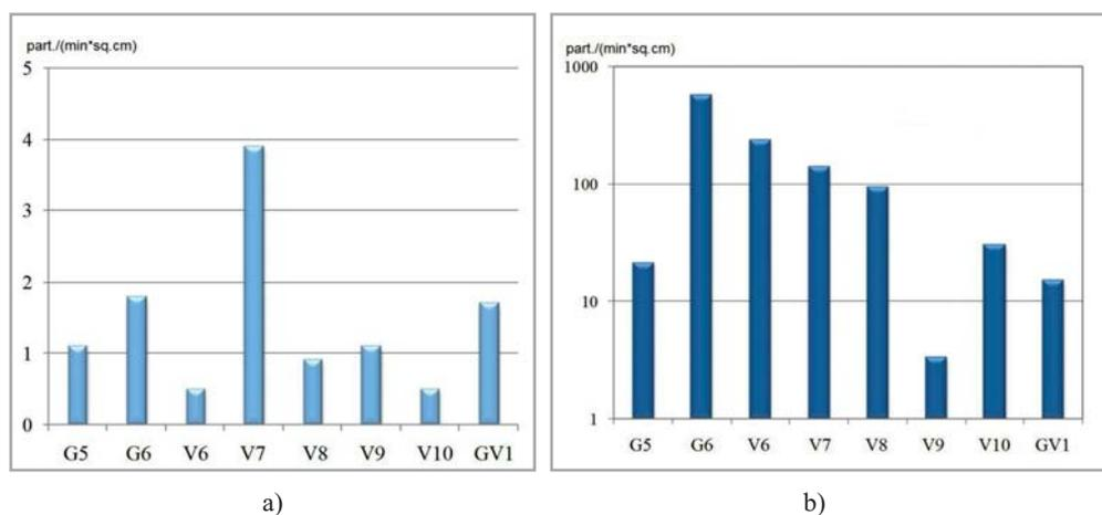
**Figure 2.** Maximal values of the density of the flux of  $\alpha$ -particles (a) and  $\beta$ -particles (b) by the results of the tunnel inspection in 1999.
