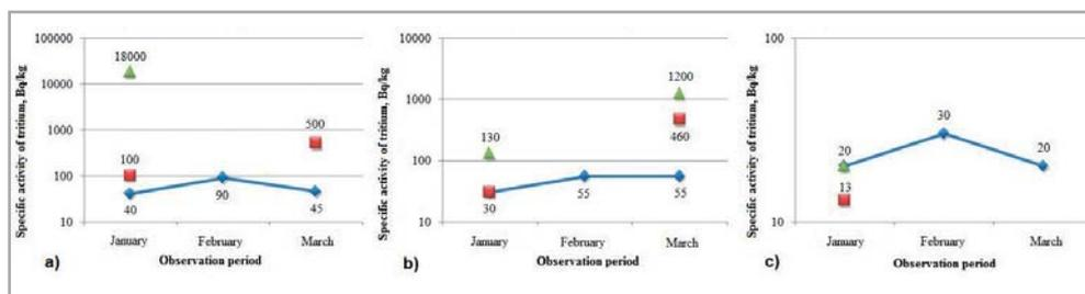
**Figure 7.** Dynamics of tritium concentration in the snow cover on the Uzynbulak stream: a) in the stream bed, b) at a distance of 50 m from the stream bed, c) at a distance of 300 m from the stream bed.
