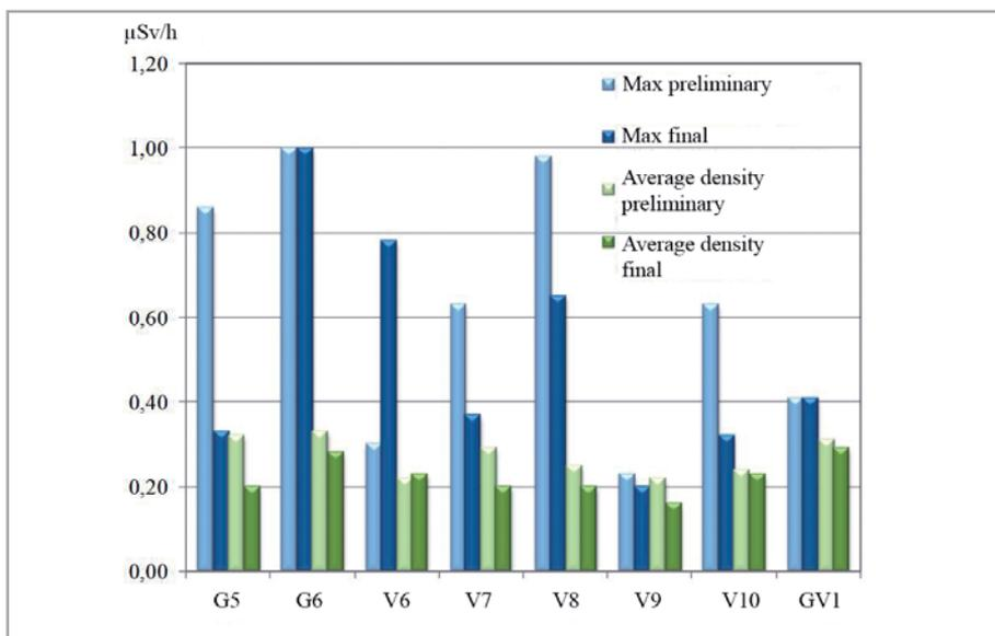
**Figure 43.** Maximal EDR values and average EDR density registered in the preliminary and final tunnel inspections
