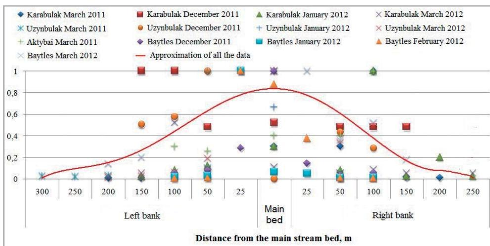
**Figure 9.** Spatial tritium distribution in the snow cover as a function of the distance from the stream beds of the studied streams normalized to the maximal value of tritium concentration
