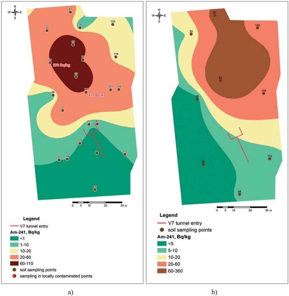
**Figure 35.** Schematic maps of  $^{241}\text{Am}$  distribution on the territory of the near-portal area of tunnel V7 during preliminary (a) and final (b) inspections
