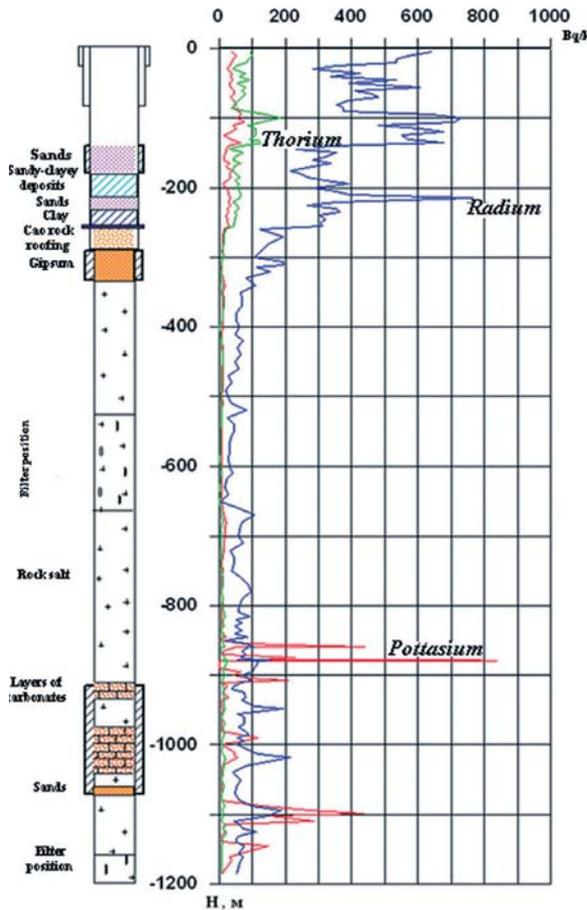
Figure 24. Gamma spectrometry at the borehole KN-12
