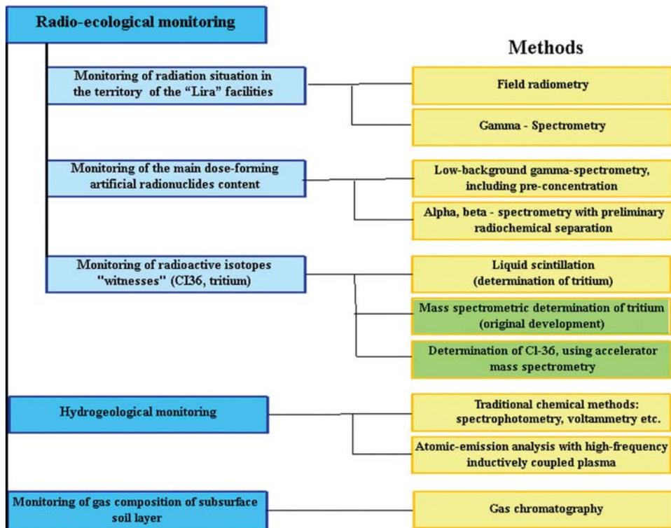
Figure 29. Comprehensive monitoring system of LIRA facilities
