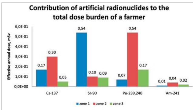
**Figure 29.** Contribution of artificial radionuclides into expected annual effective dose of a farmer through major exposure pathways in Zones I, II, III of "Baitemir" field
