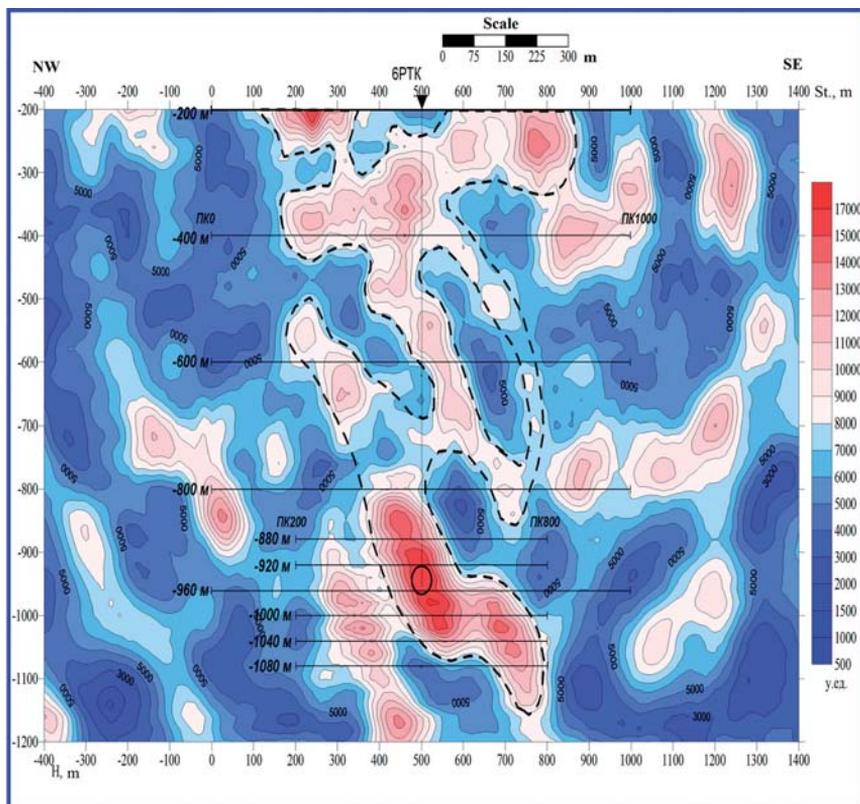
Figure 27. Deconsolidation zone in the vicinity of the cavity TK-6
