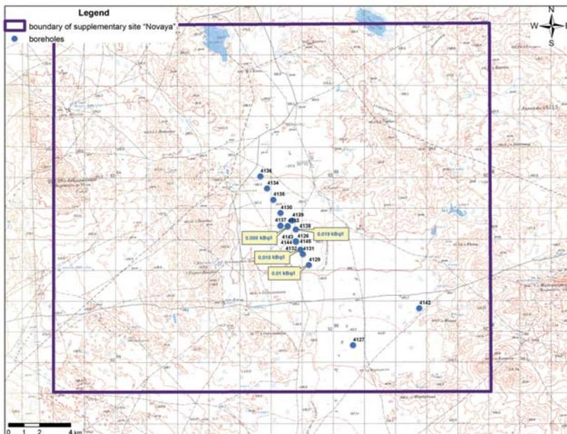
Figure 28. A scheme of location of observational boreholes on the "Novaya" site
