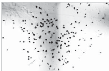
Figure 116. A fragment of a detector, exposed over the 500-250 \mu\text{m} fraction of soil sample taken at the trace from the 1953 thermonuclear explosion
